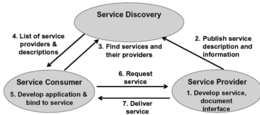
Fig. 1. Overview of roles in Service-Oriented Architecture (SOA). [4]
